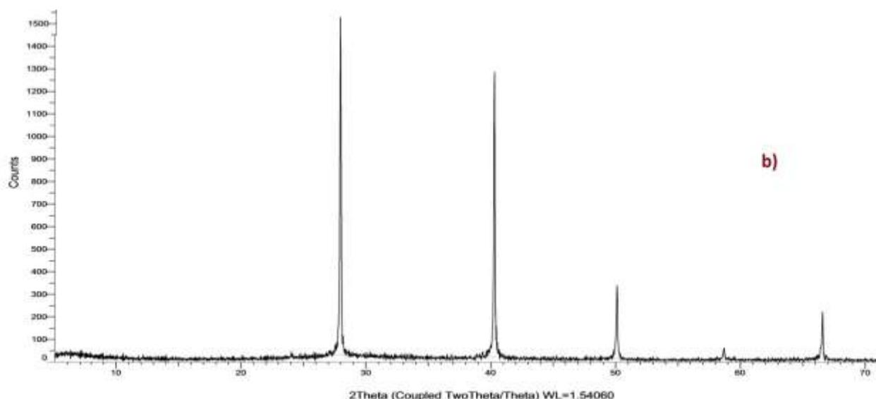
**Fig.3.** Powder X-ray patterns of alloy with composition of 70 mol% PbTe: a) a sample from the 1<sup>st</sup> series; b) a sample from the 2<sup>nd</sup> series
