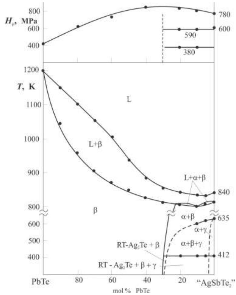
**Fig.2.** Phase diagram and concentration dependence of microhardness for the PbTe-"AgSbTe<sub>2</sub>" system
