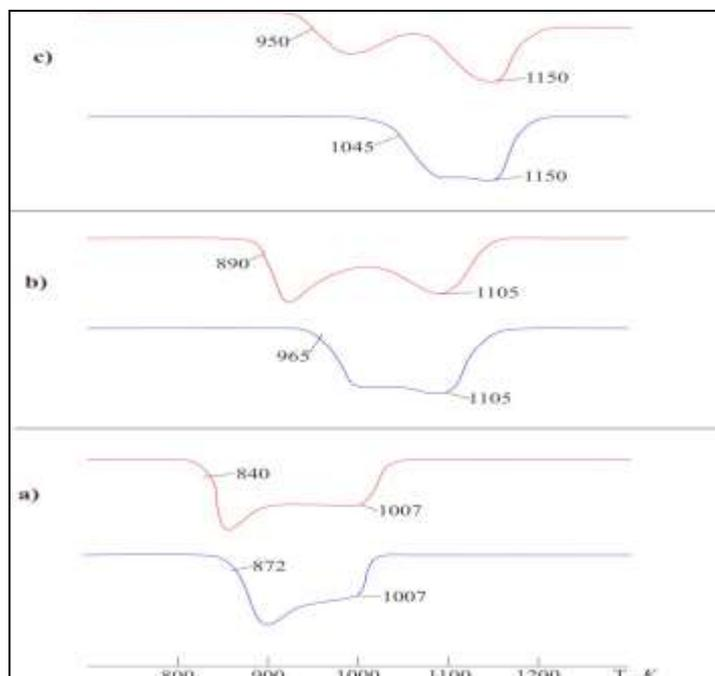
**Fig.1.** Fragments of the DTA curves for the  $\text{PbTe}$ -“ $\text{AgSbTe}_2$ ” system alloys with the compositions 60 (a), 80 (b) and 90 (c) mol%  $\text{PbTe}$ . DTA curves for samples from the 1st series are red, and those from the 2<sup>nd</sup> series are blue.
