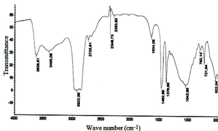
Fig. 2. IR spectrum of starting montmorillonite
