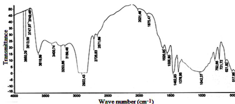
Fig. 3. IR spectrum of montmorillonite treated with octadecylamine of acetate
