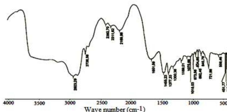
Fig. 5. IR spectrum of polyvinylpyrrolidone/organo-bentonite nanocomposite
