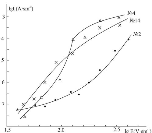
**Fig. 5.** Volt-ampere characteristics (VACH) for alloys of the  $(3\text{Bi}_2\text{O}_3 \cdot 5\text{B}_2\text{O}_3)_{100-x} - (\text{Nd}_2\text{O}_3 \cdot 3\text{B}_2\text{O}_3)_x$  system. N2-x = 10 mol%; N4-x = 20 mol%; N14-x = 70 mol%
