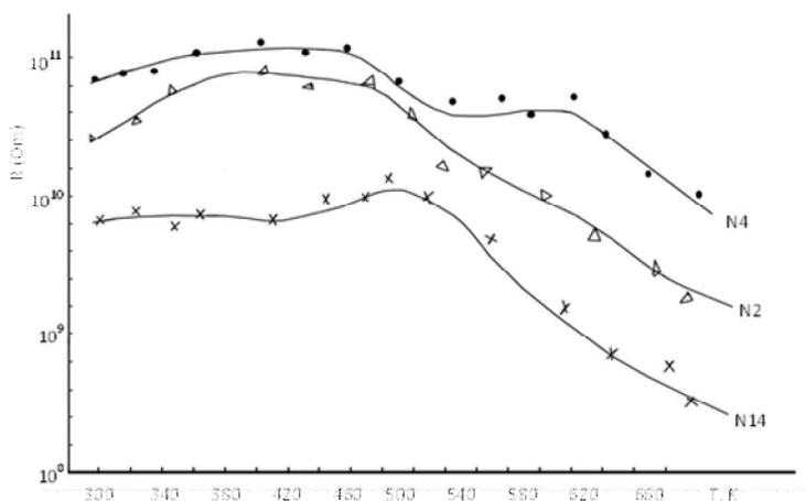
**Fig. 3.** Temperature dependence of electric resistance of  $(3\text{Bi}_2\text{O}_3 \cdot 5\text{B}_2\text{O}_3)_{100-x} \cdot (\text{Nd}_2\text{O}_3 \cdot 3\text{B}_2\text{O}_3)_x$
