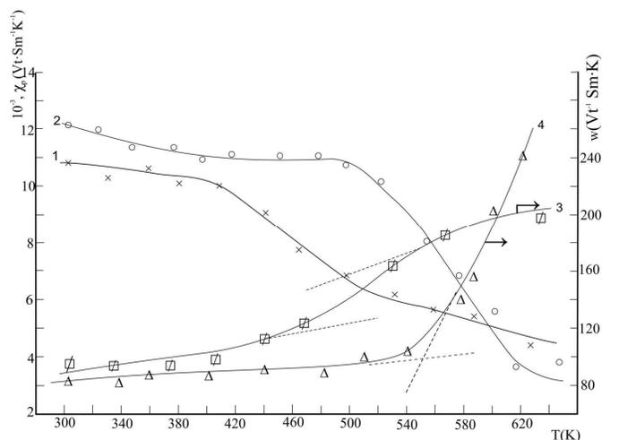
**Fig.6.** Temperature dependences of thermal conductivity (1.2) and heat resistance (3.4) in the  $(3\text{Bi}_2\text{O}_3 \cdot 5\text{B}_2\text{O}_3)_{100-x} - (\text{Nd}_2\text{O}_3 \cdot 3\text{B}_2\text{O}_3)_x$  system. 1 and 3 -  $x=50$  mol%; 2 and 4 -  $x=30$  mol%
