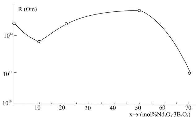
**Fig. 2.** Structural dependence of electric resistance (R) of the  $(3\text{Bi}_2\text{O}_3 \cdot 5\text{B}_2\text{O}_3)_{100-x} \cdot (\text{Nd}_2\text{O}_3 \cdot 3\text{B}_2\text{O}_3)_x$  system  $T= 300\text{K}$
