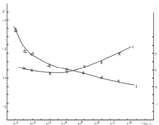
**Fig. 4.** The dependence of dielectric permittivity ( $\epsilon$ ) (1) and dielectric loss ( $\text{tg}\delta$ ) (2) of 30 mol%  $(3\text{Bi}_2\text{O}_3 \cdot 5\text{B}_2\text{O}_3)$  + 70 mol%  $(\text{Nd}_2\text{O}_3 \cdot 3\text{B}_2\text{O}_3)$  sample on dielectric space frequency.  $T=300\text{K}$ .
