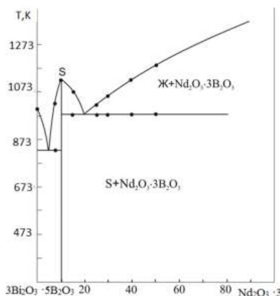
**Fig. 1.** Phase diagram of the  $3\text{Bi}_2\text{O}_3 \cdot 5\text{B}_2\text{O}_3 - \text{Nd}_2\text{O}_3 \cdot 3\text{B}_2\text{O}_3$  section.
