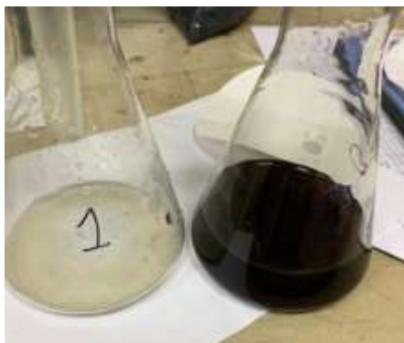
Fig. 5. Tbilisi landfill leachate water before treat (right) and after treat (left) by means of mixed carbon sorbent from polypropylene MSW fraction (1g sorbent/50ml leachate, 24 hours under static conditions).
