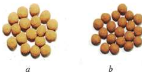
Fig.2. Pictures of granules: a - granules rounded with powder, c - granules rounded additionally without powder.
