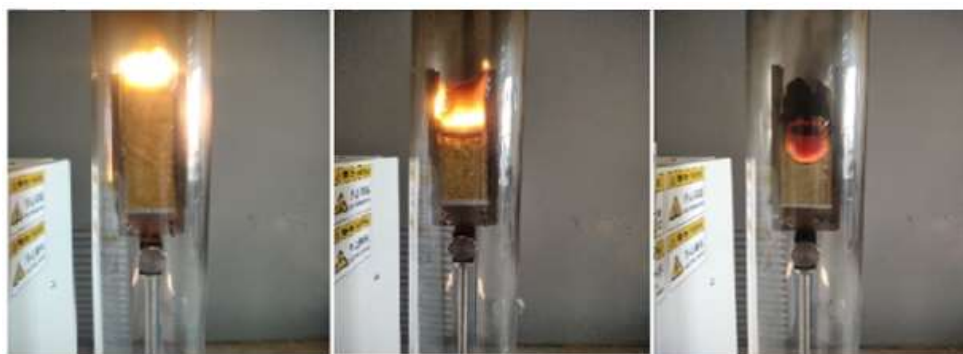
Fig. 9. Procedure for determination of oxygen index of modified textile materials
