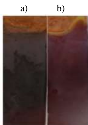
Fig. 3. Images of Cu plates with Cu 2 O deposited: (a) at the anode, and (b) at the cathode of the H-cell.
