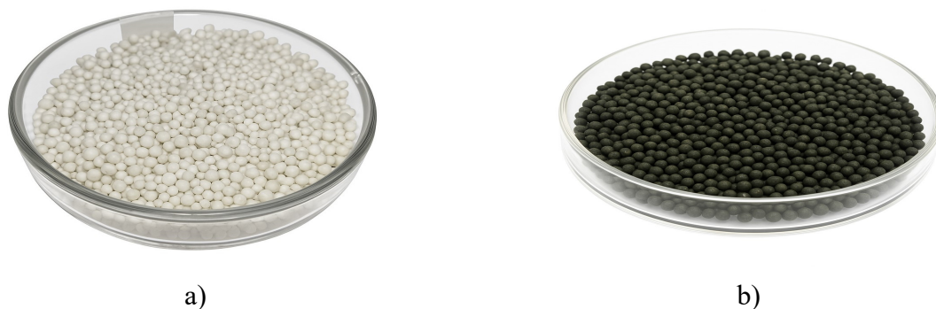
Fig. 5. Visual comparison of unmodified ammonium nitrate granules (a) and serpentinite-modified AN–SP (100:20) granules (b)
