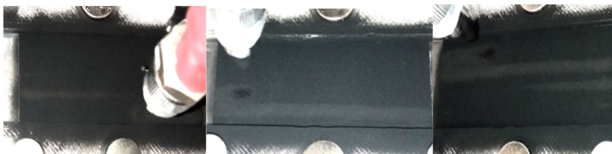
Fig. 8. Image of the spray track at different flow rate values: 54 (left), 81 (center), and 108 µl·min -1 (right).
